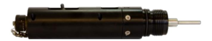
Compatible with ALL MWD Surface Systems, Rhino Mechanical Transducers offer pulse testing in linear drive pulsers used in measurement while drilling tools. With its rugged and easy to use design, the Rhino Mechanical Transducer will thread onto bottom mount pulsers allowing the technician to measure physical servo poppet movement of a linear drive pulser and deliver the pulse signal that can be decoded by MWD surface systems.
